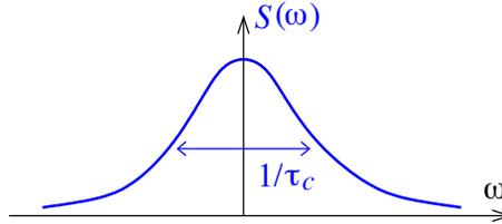
Figure 17: **Wiener-Khintchine theorem** : *width of noise spectrum is inversely proportional to the correlation time  $\tau_c$  of the process ( $\tau_c$  is the width of  $C(\tau)$ ).*
