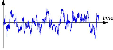
Figure 2: A realization of the Ornstein-Uhlenbeck process  $v(t)$  defined by (1.3) when  $\xi(t)$  is a Gaussian white noise.
