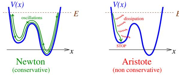
Figure 4: The dynamics described by the Newton equation conserves the energy, whereas the energy is dissipated during the "Aristote dynamics".
