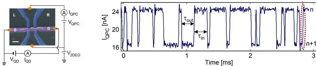
Figure 10: *A physical realization of the random telegraph process : the charge inside a quantum dot is measured as a function of the time with a neighbouring probe. The current  $I_{QPC}$  through the probe is proportional to the number of electrons inside the central island, which fluctuates by one unit (one electron). From Ref. [16].*
