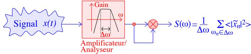
Figure 15: *Measure of the noise : the signal is amplified, duplicated and multiplied by itself. The result is averaged over a long time  $T$ .*
