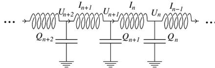
We consider harmonic solutions  $I_n(t) = \tilde{I}_n e^{-i\omega t}$ . We recall that the impedance of the capacitance is  $Z_C = 1/(-i\omega C)$  and that of the inductance  $Z_L = -i\omega L$ , where  $\omega$  is the frequency.
