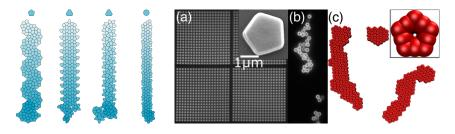
Left: One-dimensional aggregates formed by identical particles (shown at the top) that cannot fit together to tile the plane unless deformed. Right: Our fluorescent 3D-printed particles (a) arranged in a regular array after printing and before detachment from the substrate and (b) after aggregation and their (c) numerical counterparts. Insets show individual particles.
