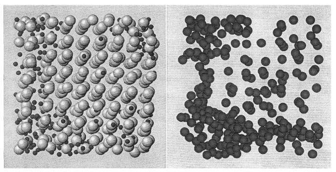
Figure 3. The left hand panel shows the arrangement of large (yellow) and small (red) spheres in the last configuration of the molecular dynamics simulation. For convenience, the radii of each species have been drawn half their actual value. The right hand panel shows the small spheres full-size and the large spheres are omitted.
