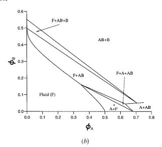
Figure 1. (a) P - X phase diagram of a binary mixture of hard spheres with a diameter ratio  $\alpha = 0.414$ , (b) Constant volume diagram: the lines indicate boundaries of two or three phase regions. Note that the ordinate in (a) is  $x_A^{1/3}$ . The star marks the phase point used as the starting point of the MD run.
