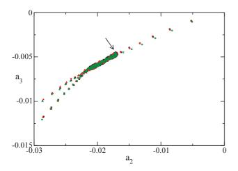
FIG. 3. (Color online) Same data as in Fig. 1, where the coefficient  $a_3$  is shown as a function of  $a_2$ . In addition to Maxwellian and asymmetric, flat initial conditions are also shown. The arrow indicates the steady state values.
