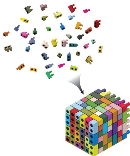
Figure 2 | Schematic of the self-assembly of 'DNA bricks' (each of which is a 32-base string of single-stranded DNA that can bind to four neighbouring bricks) into a complex structure where every brick is distinct and has a unique position. Figure reproduced with permission from ref. 15, © 2012 American Association for the Advancement of Science.
