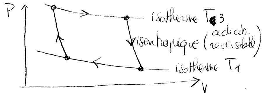
$$\gamma_c = 1 - \frac{T_1}{T_3} = 1 - \frac{b}{a^{\delta}} = 0,862$$
