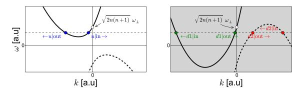
Figure 9: Sketch of the typical dispersion relations of a transverse mode in the subsonic (left plot) and supersonic (right plot) case. The horizontal dashed line is fixed by the chosen value of  $\omega$ .
