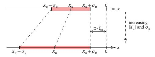
Figure 3: Schematic representation of the behavior of the parameters  $X_u$  and  $\sigma_u$  of the window function  $\Pi_u(x)$  defined in Eq. (16). The shaded zone is the region where the window function notably differs from zero. The spacing between  $X_u + \sigma_u$  and the origin is large compared to  $\xi_u$ , and this ensures that the Fourier analysis, which is made local thanks to the window function, is performed in the deep subsonic region.
