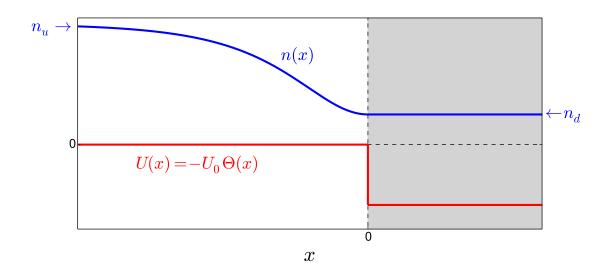
Figure 1: Waterfall configuration. The flow is incident from the left with an asymptotic density  $n_u$  and a (subsonic) velocity  $V_u$ . The downstream (x > 0) velocity  $V_d$  is supersonic. The downstream density  $n_d$  is constant and lower than  $n_u$ . The region x > 0 is shaded in order to recall that it corresponds to the interior of the black hole.
