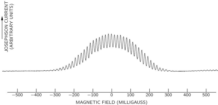
Fig. 21-8. A recording of the current through a pair of Josephson junctions as a function of the magnetic field in the region between the two junctions (see Fig. 21-7). [This recording was provided by R. C. Jaklevic, J. Lambe, A. H. Silver, and J. E. Mercereau of the Scientific Laboratory, Ford Motor Company.]
