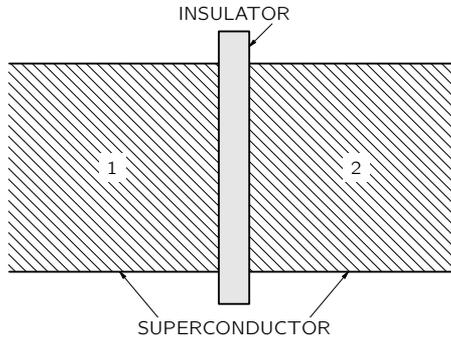
Fig. 21-6. Two superconductors separated by a thin insulator.
