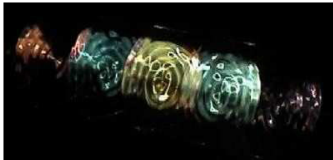
Figure 6. Close-up of soap films subject to a standing sound wave. The central film is located at an antinode. The error on the relative position of the film with respect to the antinode is equal to the spacing between the films, that is 1 cm. The colour of a film corresponds to a certain film thickness which increases with the amplitude of the standing wave. Here the frequency of the sound wave was 670 Hz. According to equation (2), this corresponds to n = 8 with c = 340 \text{ m s}^{-1} .
