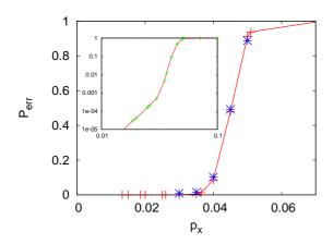
FIG. 1: +: block error in the x-channel,  $P_{\rm err}^x$ , versus the phase error probability  $p_x$ , for the code with m=12, t=4,  $M_x=1378$ . The line is a guide to the eye. Also shown is the same curve for a random LDPC code (×). The inset gives the same data in a log-log plot
