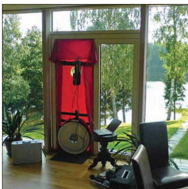
Air permeability test. Source: Tõnu Mauring
