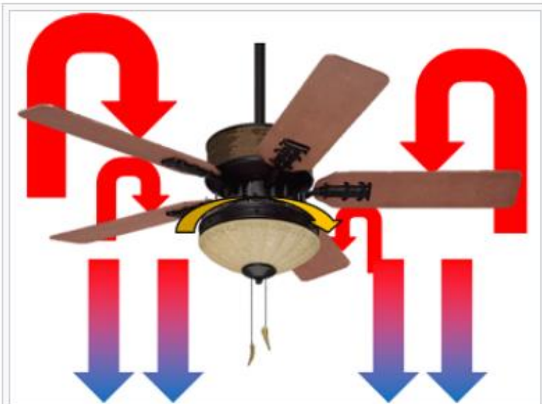
Figure 2. In the summer, ceiling fans should rotate counterclockwise to mix warm air and force a cool breeze downwards, creating a downdraft. [8]
