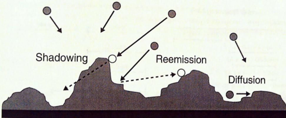
**Fig. 1.3.** Diagram of growth effects including diffusion, shadowing, and reemission that may affect surface morphology during thin film growth. The incident particle flux may arrive at the surface with a wide angular distribution depending on the deposition methods and parameters.
